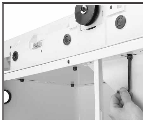
Figure 11. Securing the jointer to stand.
