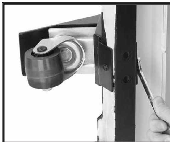
Figure 9. Bolting wheel assembly to stand.
