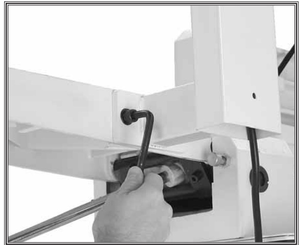
Figure 21. Attaching pedestal switch to the back of the jointer.
