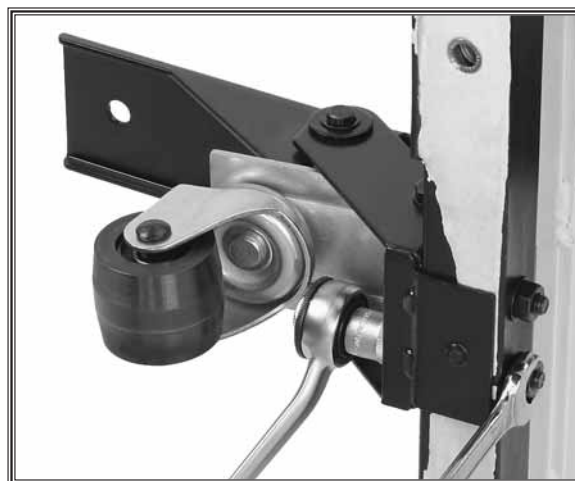
Figure 10. Securing wheel assembly to stand.
