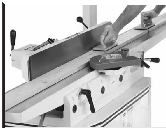
Figure 34. Typical surface planing operation.
