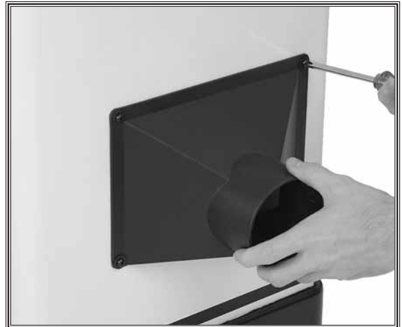
Figure 22. Attaching dust port to jointer stand.
