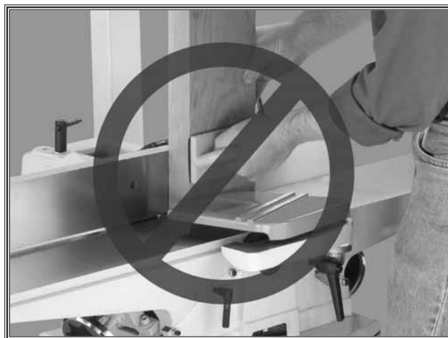
Figure 5. Never joint end grain!
