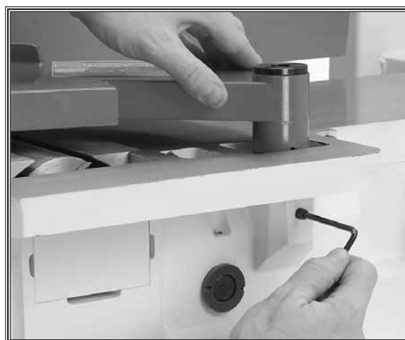
Figure 20. Securing the cutterhead guard.
