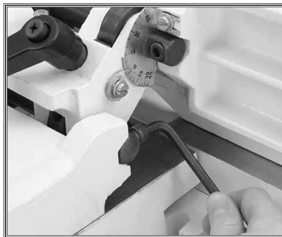
Figure 18. Attaching fence to carriage.
