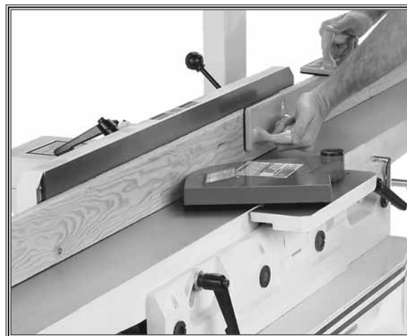
Figure 36. Typical edge jointing operation.
