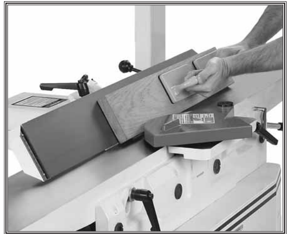
Figure 38. Typical bevel cutting operation.
