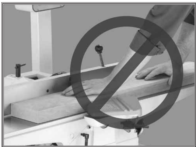
Figure 2. Never surface plane without push blocks!
